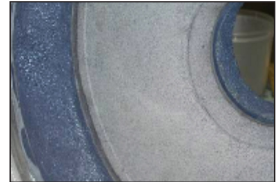
Completed application showing machined ARC surface
